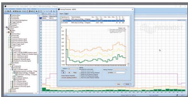
Crosshead vibration threshold setting per segment
